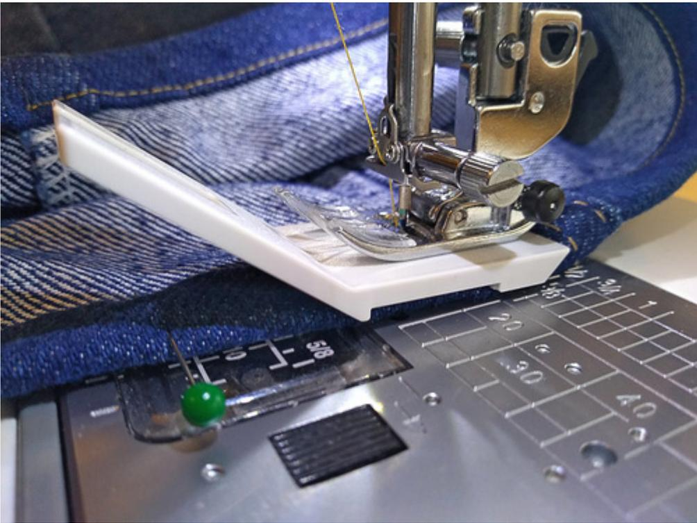
Stop and remove the hump jumper, then continue sewing to complete the hem.
