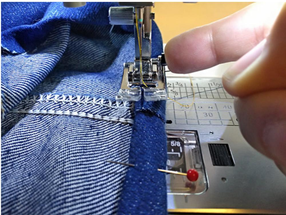
Still holding the button, lower the foot. The button will hold the foot in position parallel to the bed of
