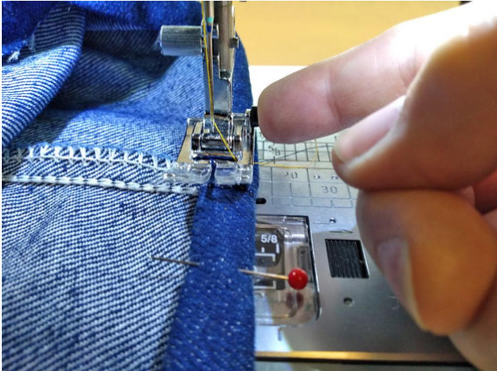
Start stitching. As the machine moves forward, the button will release. You will glide up and over this first thick seam.
