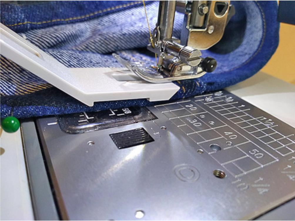
Continue sewing until the foot is completely past the bulk of the seam.
