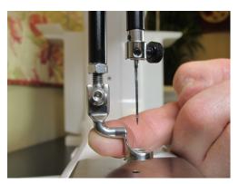
3. Ensure the foot is centered with the needle when the foot is fully tightened with the 2.5mm hex wrench. If it isn't properly centered, loosen the lock nut; center the foot with the needle; hold the foot in position; and firmly tighten the lock nut.
