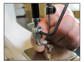
NOTE: We recommend that you use the 1.5mm couching foot to ensure the foot is centered over the hole in the needle plate. Then slowly rotate the hand wheel to confirm that the needle smoothly cycles through the center of the hole. Then put on each of the other two couching feet and manually cycle the needle through the hole.
