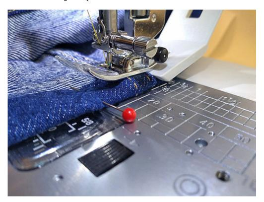
Stop, and with the needle down, raise the foot. Remove the hump jumper from the rear of the foot and re-position it under the front of the foot. Lower the foot. The foot should again be level and parallel to the bed of the machine.
